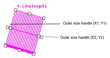
To change the width of the line to be inspected, drag one of the outer size handles away from or toward the center of the line.
