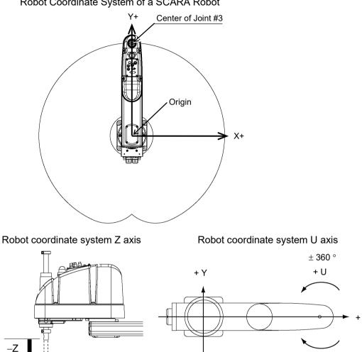
Robot Coordinate System of a SCARA Robot
