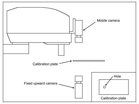
Mobile Camera Calibration using Fixed Upward Camera
