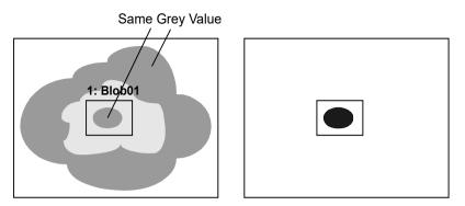
Figure C: Scene that cannot be segmented by gray-scale value
