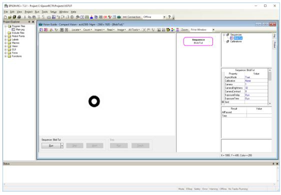
The Vision Guide window with target feature in center of image display
