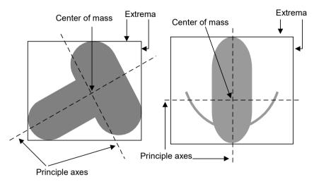
Principle axes, center of mass, and Extrema
