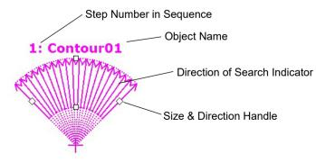
New Contour Object Layout (ContourMode:Arc)
