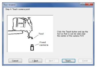
Jog the robot so that the target object can be detected near the center of camera's FOV.
