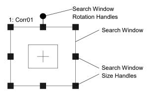
The size of the search window is very important when configuring a vision object. The larger the search window, the more time will be required to process the search. It is a good idea to make the search window large enough to handle the variation in part position while keeping it as small as possible. Sometimes the use of *6.2.10 Frame object* can help reduce the size of search windows.
