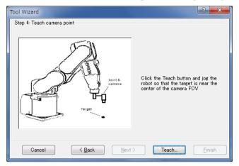
Jog the robot so that the target object can be detected near the center of the field of view.
