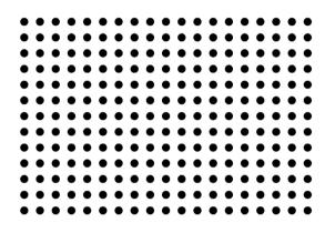
It is important to set the square lattice pattern so that it fills the entire field of view of the camera. If calibration is performed while the lattice pattern is in only a part of the field of view, distortion cannot be corrected properly since the area with no lattice pattern is not taken into account.
