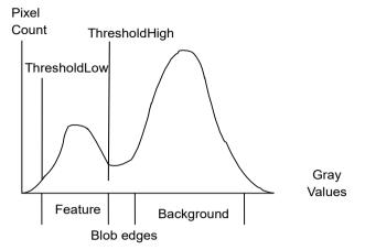
Setting the threshold values using a histogram
