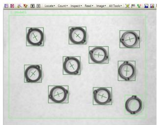
Image of 10 Rings with Improved Threshold Settings
