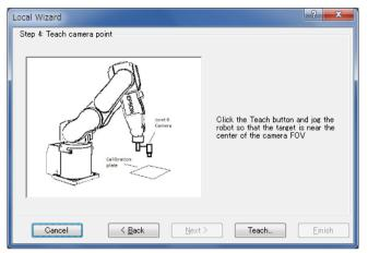
Jog the robot and move the center of the calibration plate to the center of the field of view.
