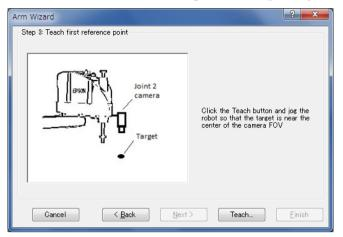
Jog the robot so that the target object can be detected near the center of camera's FOV.
